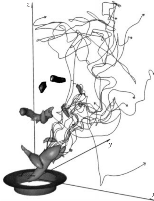
FIGURE 8. Vortex lines through the hanging vortex. Isosurface of pressure at \bar{p} = -3.6 included to show locations of structures.
