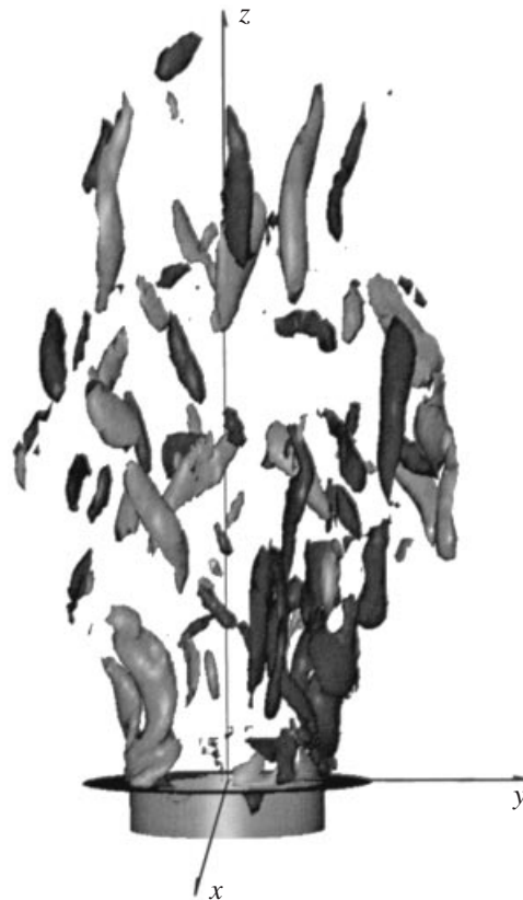
FIGURE 10. Isosurfaces of vertical vorticity, back view. Light grey surface value: +20, dark grey surface value: -20. Direction of crossflow is out of the page.
